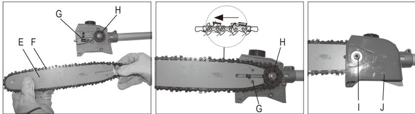
**Important!** Do not fully tighten the fastening screw until after you have adjusted the chain tension.
