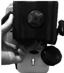
2. Turn the engine switch to the ON position.
