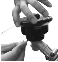
**c) Release the Nylon cutting head.** Use screw driver to hold flange and then rotate the Nylon cutting head clockwise, it will be replaced.
