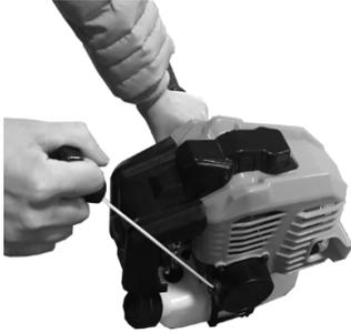
7. When the engine is running and idling, the throttle lever on handle is as below picture. First press the lock off lever and then switch the throttle lever on, the machine will be working.
