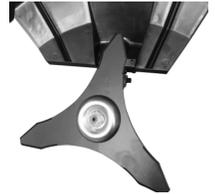
**e) Release blade.** Use screw driver to hold flange and release nut, the blade can be took off.
