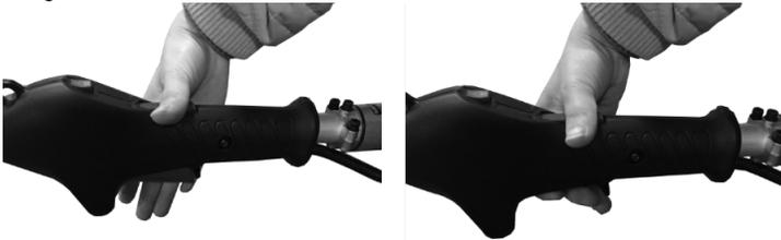
8. Adjusting line length when working: This machine is fitted with a "Tap & Go" head. To release more line, tap the cutting line head against the round with engine at top speed: the line will be released automatically and the knife cut off the excess length.
