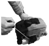
5. Pull the starter grip slowly for 10 - 15 cm until you feel some resistance, then tug it a few times until you hear the engine turn over. Then adjust the choke lever to (ON) position.
